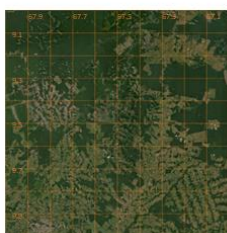
Fig. 8 Example of operational accuracy improvement by v4.2 grid-refinement in tile S09W063 at the beginning of the rainy season in November 2024. Whilst v4.1 processed TS statistical parameters over the entire 1°x1° tile, v4.2 performs calculations at a 100-fold finer resolution, resulting in substantial reduction in false alarms and omission errors.
